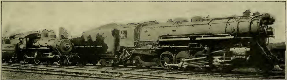
MIKADO 2-8-2 TYPE LOCOMOTIVE NO. 8600, OF THE MICHIGAN CENTRAL, SAID TO BE THE MOST POWERFUL OF ITS WEIGHT AND ON THE LEFT, ENGINE NO. 8977, FORMERLY 248, STILL RUNNING AFTER A SERVICE OF FORTY YEARS
